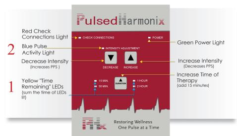
Press the **Duration** button to set one of the 15 therapy durations lengths. Each button press adds an additional 15 minutes.
